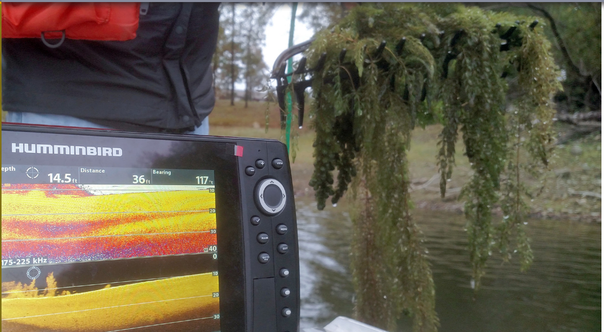
Traditional and down-imaging sonar images of coontail, left, with actual coontail collected by a weed collection rake from the same location at DeGray Lake, right.
